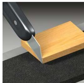
Figure 5: To accommodate setting blocks, notch out tape
